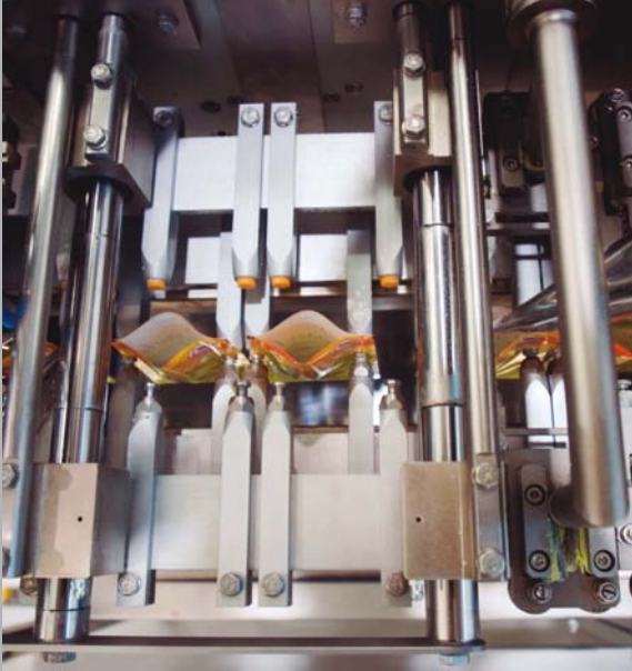
Dosing station top view.
