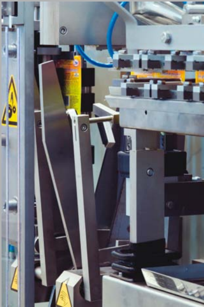
Scissor for pouch cutting, and film pulling by means of a servomotor.
